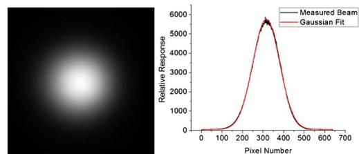
Fig. 3. SWIR camera image of the beam at 25.7 W SC (left). Corresponding Gaussian fit of the beam cross section at 25.7 W (right).
