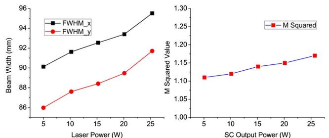
Fig. 4. Measured FWHM beamwidth with power scaling (left). Corresponding  $M^2$  values with power scaling (right).
