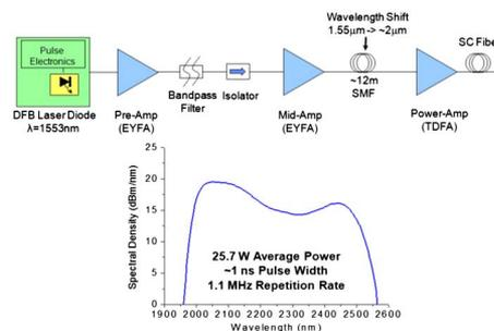
Fig. 1. Optical layout of the 25.7 W SC laser (top). 25.7 W SC output spectrum from 1.95 to 2.55  $\mu\text{m}$  (bottom).
