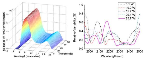
Fig. 5. Sixty scan sequence of the 25.7 W SC spectra (left). SC output relative variability with power scaling (right).
