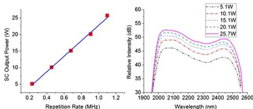
Fig. 2. Linear scaling of SC average power with repetition rate (left). Nearly constant SC output spectra with average power scaling (right).
