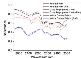
Fig. 6. Diffuse spectral reflectance measurements using the SC laser (solid) and lamp reference measurements (dashed).
