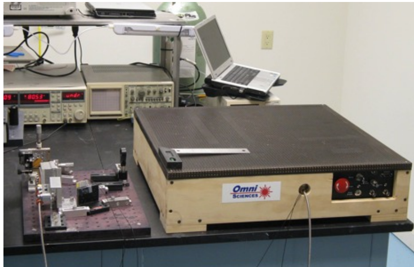
Figure 2: 64W SWIR supercontinuum laser
